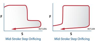
Velocity Hydraulic dampers/rate controls are velocity sensitive devices, usually expressed as  $F = CV^{\infty}$ . KYNTEC designs product to provide the exact force profile (or profiles) needed by carefully selecting fluids, orificing, and mechanical elements to perform over the
