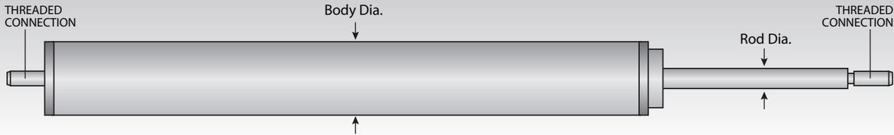
Overall length and compressed length are dependent on the stroke and mounting options selected. Contact KYNTEC Engineering for your exact dimensions. Custom stroke lengths to fit your specific application are available.
