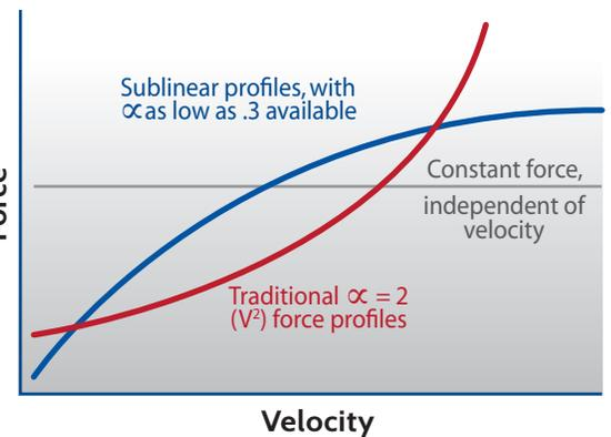
Hydraulic dampers/rate controls are velocity sensitive devices, usually expressed as  $F = CV^\alpha$ . KYNTEC designs product to provide the exact force profile (or profiles) needed by carefully selecting fluids, orificing, and mechanical elements to perform over the design operating range.
